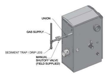
Support piping with hangers, not by the boiler or its accessories.
