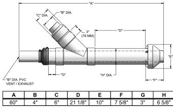
5. Install the Y concentric fitting and pipe assembly through the structure's hole from an inside wall.
