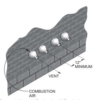
Figure 4-13 Concentric Vent and Combustion Air Termination
