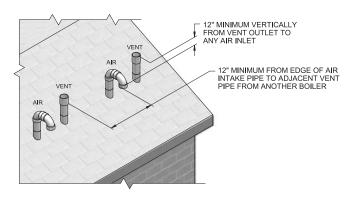
Figure 5-3 Alternate Vertical Terminations with Multiple Boilers
