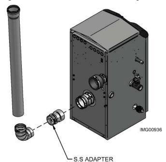
\*Use of FasNSeal Flex smooth inner wall vent is to be used in vertical or near vertical sections only, taking precaution to ensure no sagging occurs of the vent system. Connect to the FasNSeal rigid vent using specially designed adapters and sealing method, see manufacturer's instructions.
