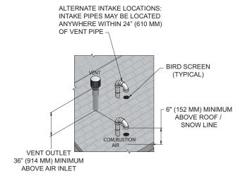
8. Locate terminations so they are not likely to be damaged by foreign objects, such as stones or balls, or subject to buildup of leaves or sediment.
