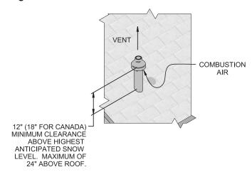
Figure 5-5 Do Not Install U-Bend to Rain Cap
