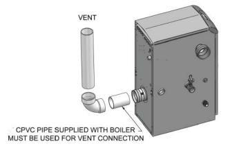
NOTE: CPVC VENT PIPE AND VENT FITTINGS MUST BE USED IN CLOSET AND ALCOVE INSTALLATIONS.
