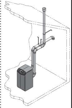
**Figure 3-5** Vertical Vent, Sidewall Air
