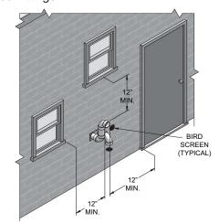
Figure 4-3A Clearance to Forced Air Inlets
