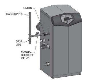
Figure 7-2 Gas Supply Piping - Model 286
