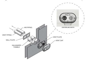
Table 4B Sidewall Vent Centerline Dimensions
