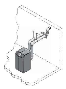
**Figure 3-1** Two-Pipe Sidewall Termination - See page 22 for more details
