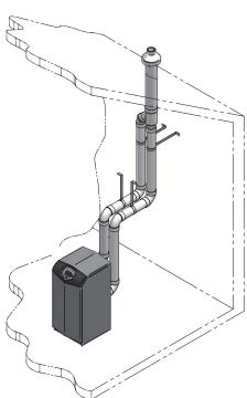
**Figure 3-4** PVC/CPVC Concentric Vertical Termination - See page 31 for more details
