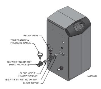
Near boiler piping components
